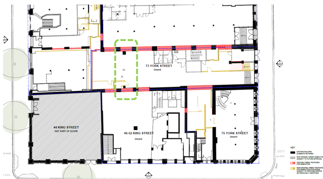
Figure 23: Excerpt of Ground Floor demolition plan. Original rear wall of 73 York Street outlined in green.
