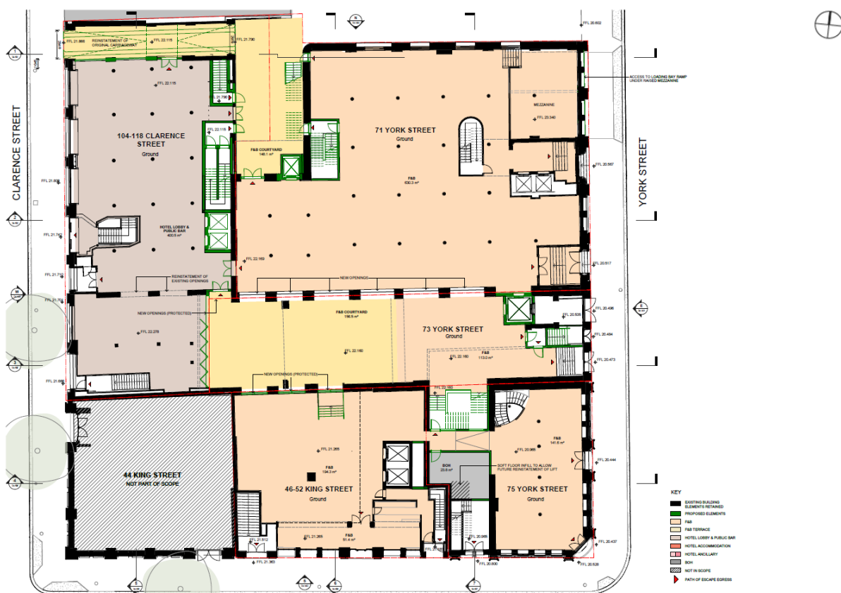
Figure 20: Proposed ground floor indicating openings to connect all buildings, reinstated northern carriageway and new central courtyard
